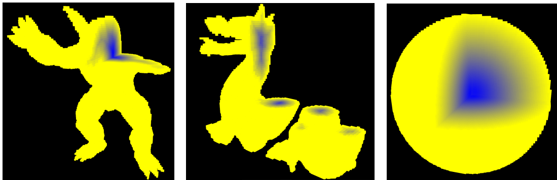
Fig. 6.1: SDF of three models. Some voxels are removed for better visualization. The magnitude of the signed distance of blue-colored voxels is larger than yellow-colored ones.
